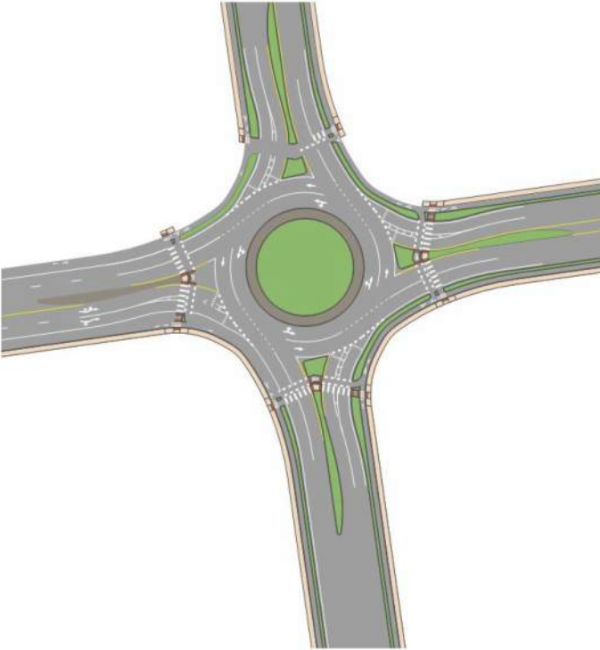
(2022) MASSDOT GUIDELINES FOR THE PLANNING AND DESIGN OF ROUNDABOUTS - 2 CIRCULATING LANES
